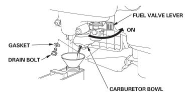
4. After draining the carburetor bowl and fuel tank, install the drain bolt and gasket, and tighten securely.
